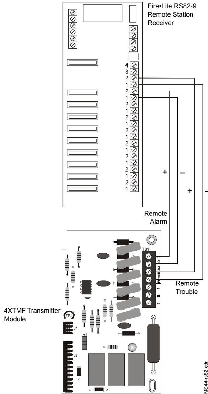
Figure 27 RS82-9 Connections
