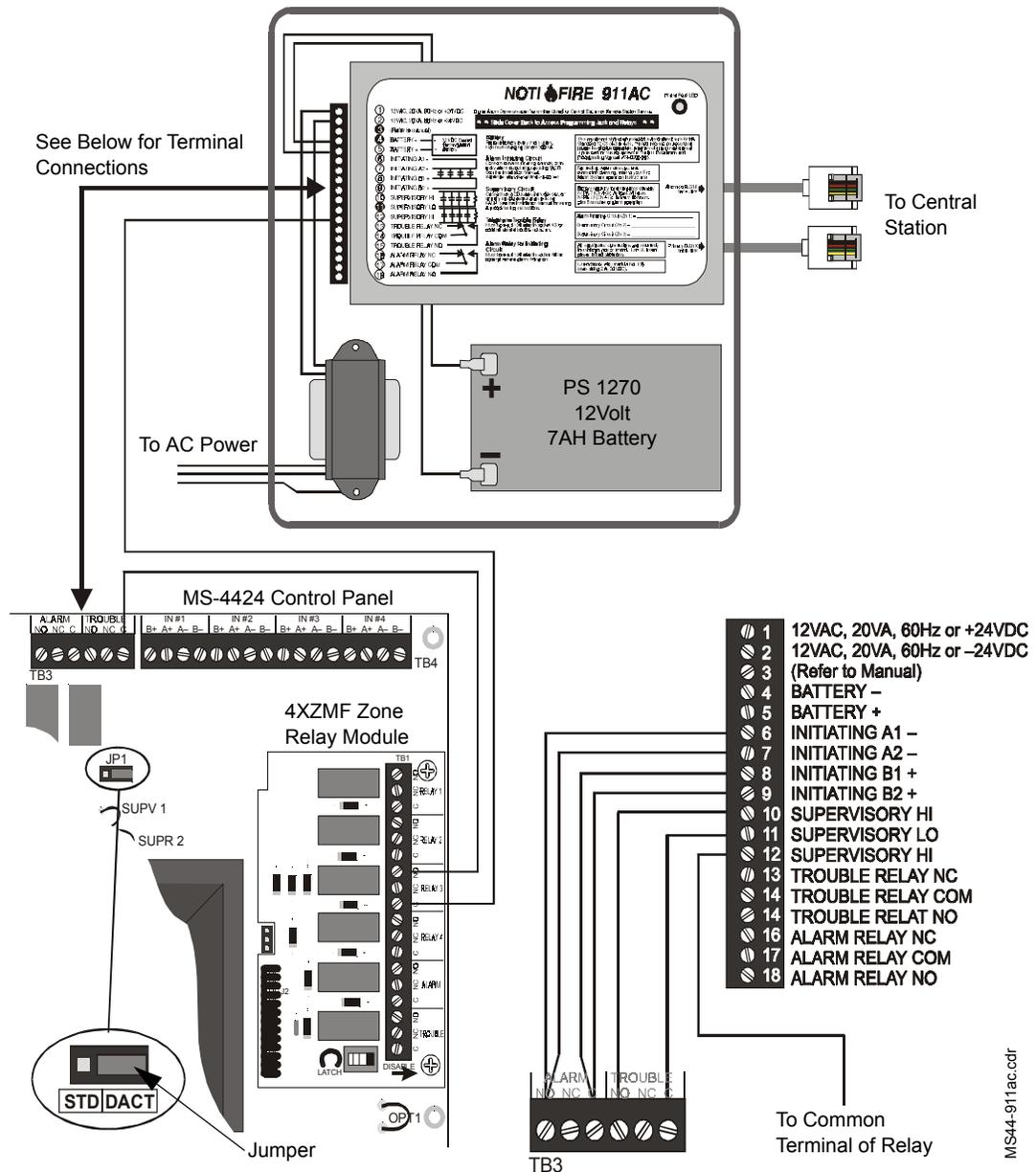
Place jumper over pins as shown when employing a DACT. This directs the control panel to transmit all trouble conditions except AC LOSS.
