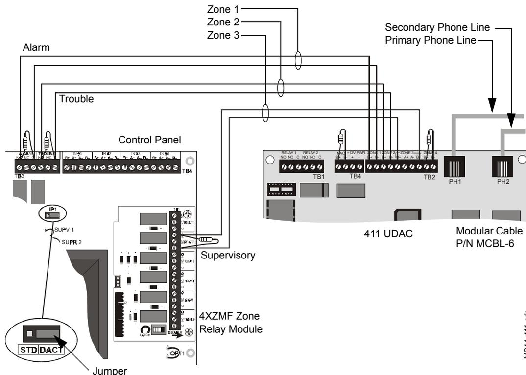
Figure 25 411UDAC Connections
