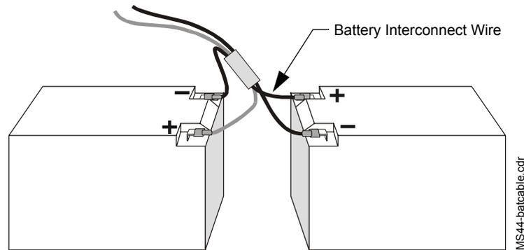
**Figure 20 Battery Connections**
