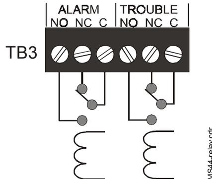
Figure 11 Schematic Representation of Alarm/Trouble Coils & Contacts
