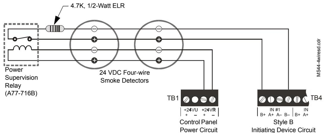
**Figure 8 Typical Connection for Four-Wire Smoke Detectors**
