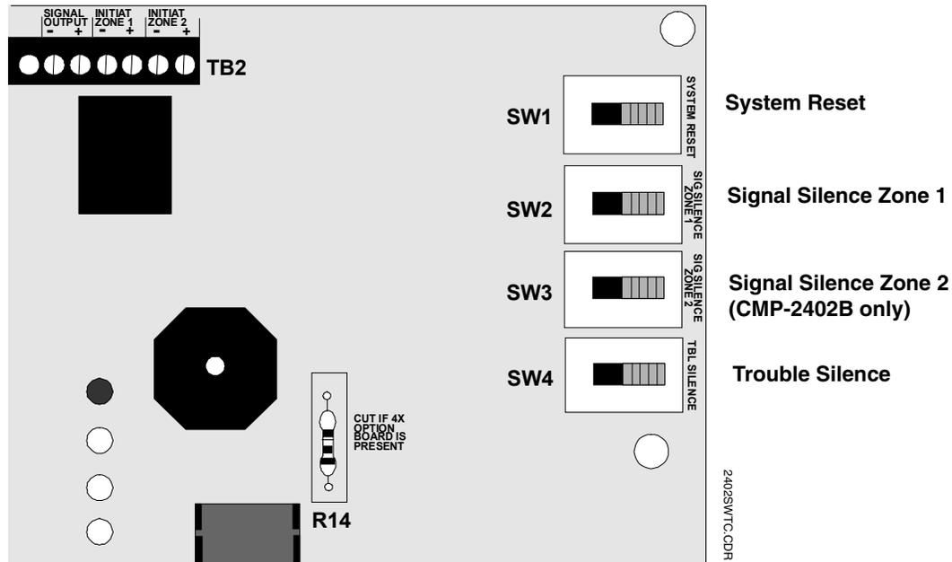
All switches are illustrated in their normal position. The function of each switch is listed below.
