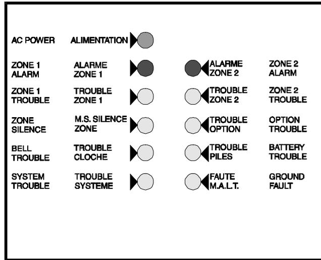
The LED indicators for the CMP-2401B/CMP-2402B are labeled in English and French. The purpose of each indicator is listed below:
